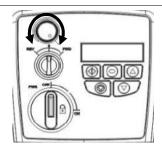
The potentiometer will control the motor shaft rotational speed.  $\label{eq:control} % \begin{center} \bend{center} \end{center} \end{center} \end{center} \end{center} \e$
