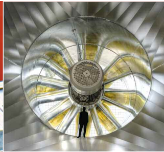
Axial fan with air flow volume and up to 150\,000\text{ m}^3/\text{h} and upstream guide vane. Application: Realistic simulation of different air flow situations.
