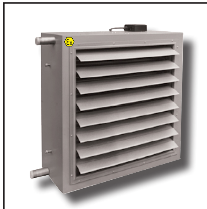
Speed controllable air heaters for steam or water. ATEX approvals for zone 1 and 2. Optional AISI316
